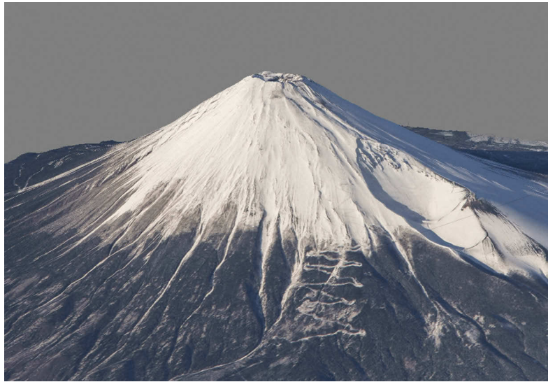
Figure 5. 3D model of Mount Fuji derived from 27 images (ISS046-E-35801 to ISS046-E-35828) taken by astronauts from the ISS. Photos alignment, dens cloud, mesh and texture generation were performed with Agisoft Metashape Professional. The 3D model was georeferenced with five ground control points. The GSD of the final model is 5 m. All ISS photos can be downloaded here: https://eol.jsc.nasa.gov .
